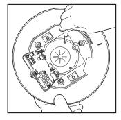
b. Unscrew the three Phillips screws located underneath the hinged door.
